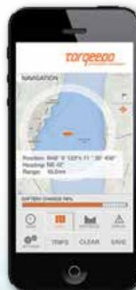
**TORQ TRAC** The dashboard for electric motors on your smartphone. Bluetooth accessory plugs in-line on the throttle cable and transmits a variety of great information to a smartphone. The App can be downloaded for free from the App store on your device.
